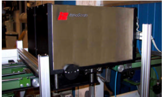
Picture 2: Two special modules side-stacked to inspect cans fed bottom-down from DRD press.
