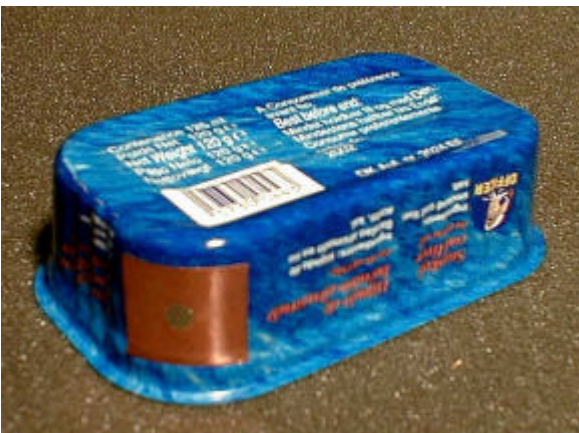
Picture 9: Can with calibrated 50 \mu\text{m} hole placed in corner.
