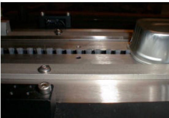
Picture 3: Belt-brush drive feeding cans to the point of inspection. (Right to left)
